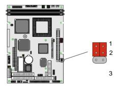
Connector : JSND Type : onboard 3-pin header
